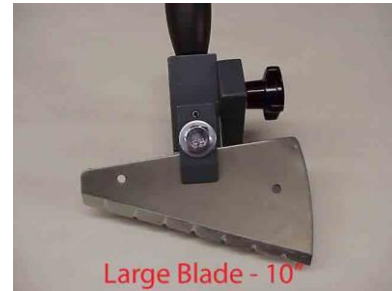
Align Pivot Bolt to the right.
