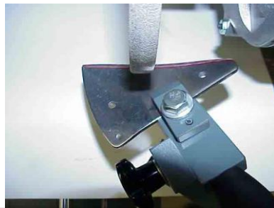
Take a light grind moving the blade across the face of the wheel from toe to heel, move smooth and steady .
