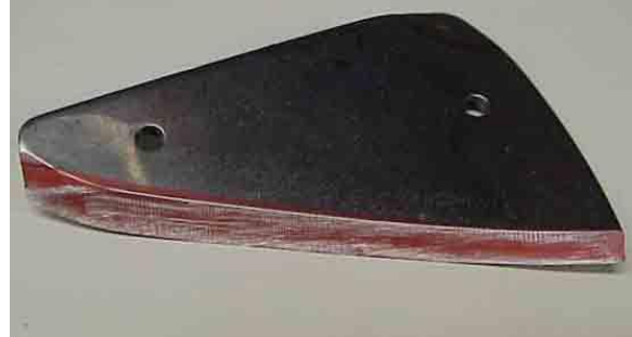
Scratch test lines should cover the grind from one end of the blade to the other.
