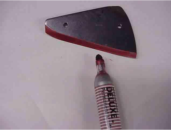
Color the grind of the blade
