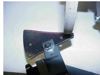
Take a light grind moving the blade across the face of the wheel from toe to heel, move smooth and steady .
