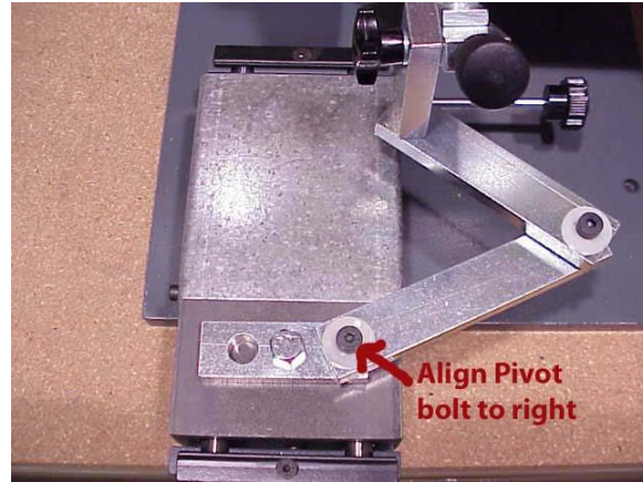
Align Pivot Bolt to the right.
