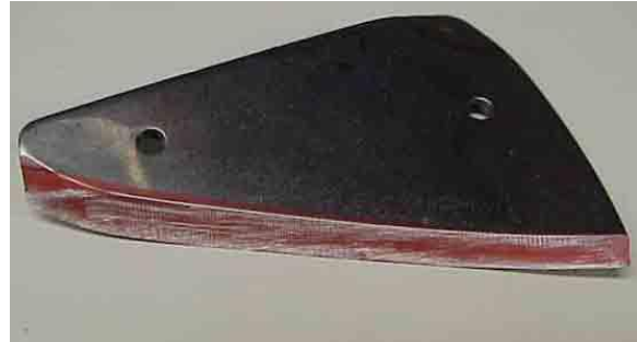
Scratch test lines should cover the grind from one end of the blade to the other.
